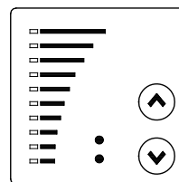
Fig. 19 Control panel of a CME pump
